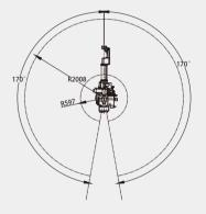
A-Way Diagram (End Flange Mounting Dimensions)
