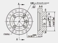
**B-Way Diagram (Base Mounting Dimensions)**
